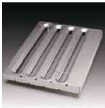
The labyrinth filters are constructed entirely from 18-10 stainless steel, they have handles for removal and can be washed in professional dishwashers. Dimensions: 40x50x4 cm.
